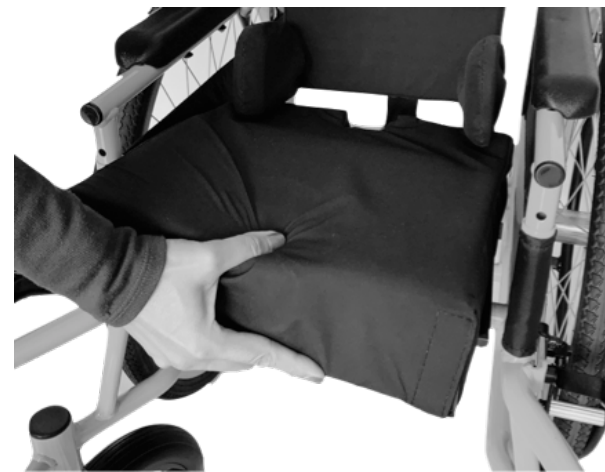
Figure 6. Placing the seat cushion correctly
