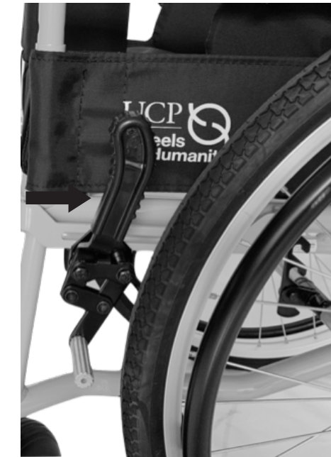
Figure 2. Wheel lock - unlocked
