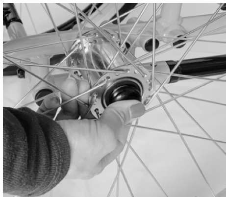
Figure 13. Quick-release button of the rear wheel axle.
