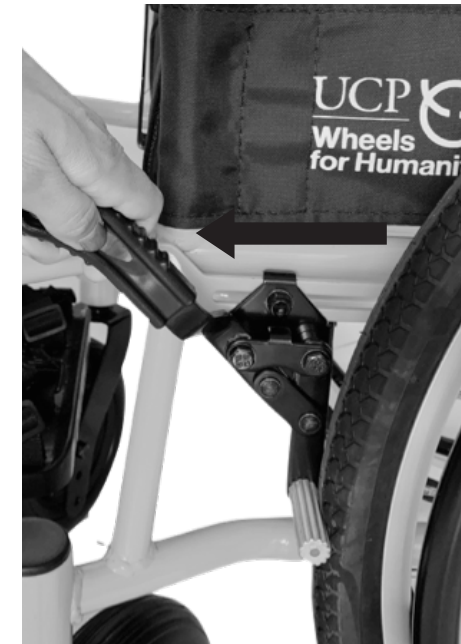
Figure 1. Wheel lock - locked
