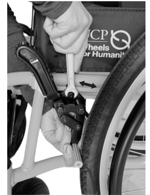
Figure 3. Adjusting the wheel locks
