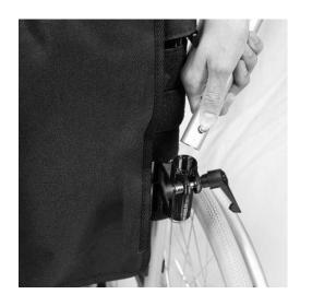
Loosen the push handle adjustment clamp. Press the spring pin on the push handle tube and insert the push handle inside the push handle adjustment clamp.
