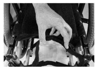
Remove the Velcro strap under the seat completely.
