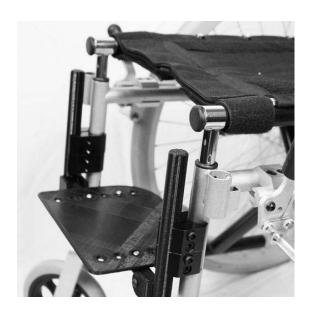
The footrest can also be adjusted horizontally. Adjust the footplate in the desired location. Tighten the footplate to the footrest tube using the fasteners provided.
