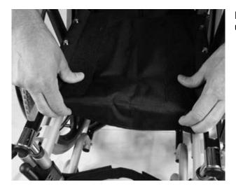
Fold the fabric at the front of the seat panel under the seat.
