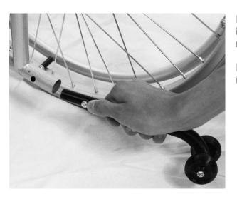
Press the spring pin on the anti-tipper tube and insert the anti-tipper inside the frame bottom rail.
