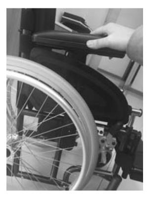
After adjusting the height and length of the side guard, insert the side guard band in the side guard mounting socket.
