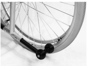
When not in use, rotate the anti-tippers up 180 degrees until the spring pin fits inside the hole in the frame bottom rail.
