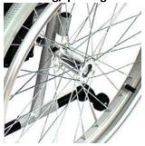
To mount the rear wheels on the frame, place the rear axle through the hub bearings and place the frame spacer on the rear wheel axle.
