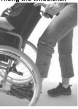
Push the bottom rail rear end down while pushing down and back on the push handles.
