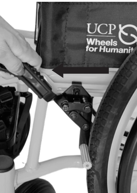
Figure 1. Wheel lock - locked
