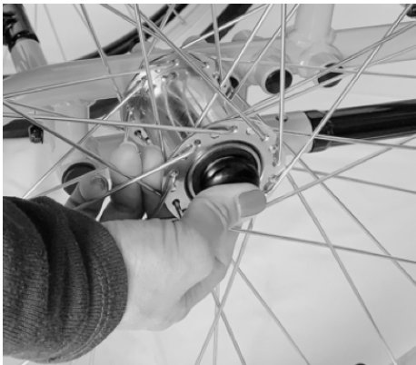
Figure 13. Quick-release button of the rear wheel axle.
