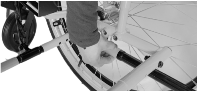
Figure 16. Anti-tipper’s pins for attachment.
