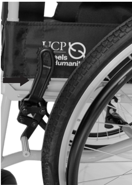
Figure 2. Wheel lock - unlocked
