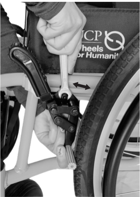
Figure 3. Adjusting the wheel locks
