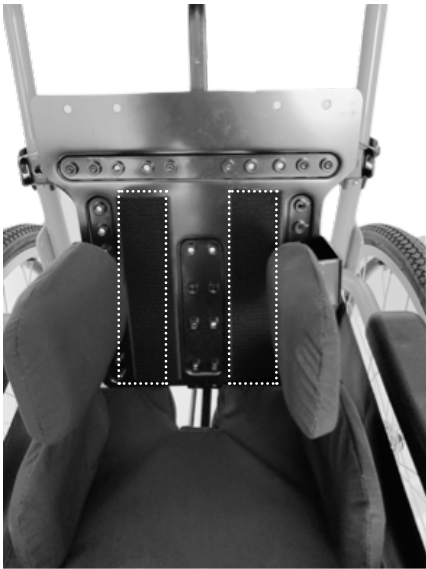
Figure 9. Backrest pan with Velcro.
