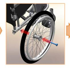
**3.** Make sure the quick release detente (ball) passes completely through the axle block so that the axle will not slide out unintentionally. Release the black button and the axle will be locked in place.
