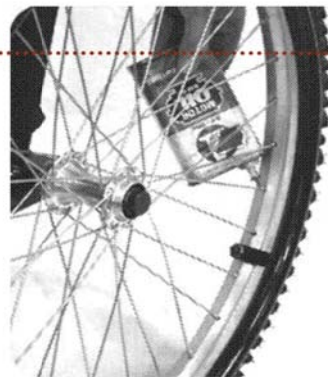
Spokes Put a tiny drop on each spoke where it enters the nipple.
