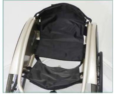
Backrest and Kneeling panel in place
